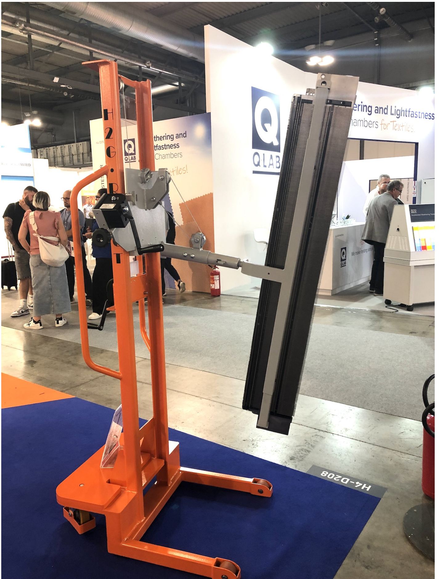
H2G Robot is a robotic lifter for removing needlebeds. © Knitting Industry
