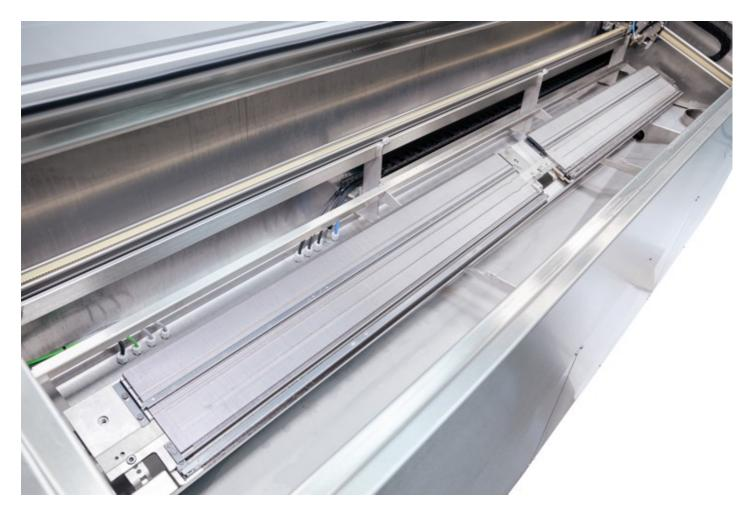
The main features that can be found in every H2G model include a digital level of the quantity of water inside the deposit, automatic drying after washing, control of the washing temperature of washing fluid, an alarm for clogged filters and dirty water, and a countdown to the end of the washing cycle.
